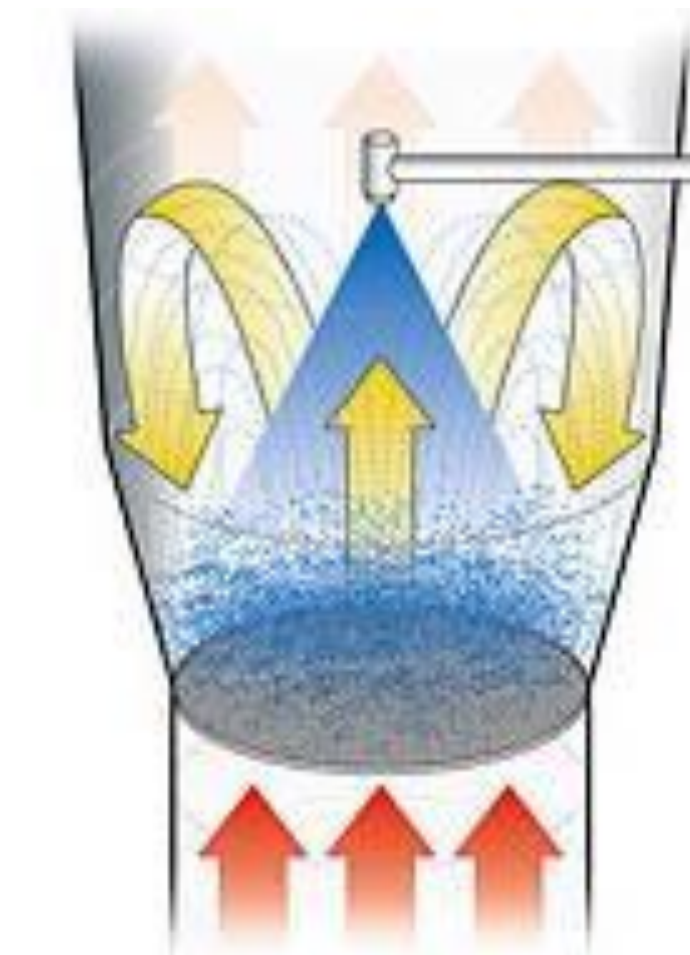
Schematic of the top-spray coating process. (Device Glatt220)
