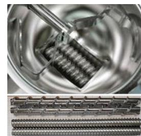
Fig.: Inside of hopper and two different screw types.
