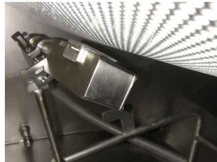
OCT Sensor in-line setup measures coating thickness and uniformity. © RCPE
